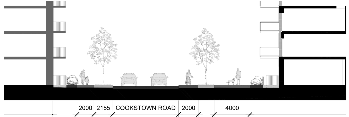
Section B – Secondary local street / through-road – Parkside street adjacent to open space with street trees
